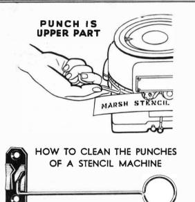
A punch clogged with paper will not cut clear thru. Brittle, low grade stencil board or cutting one line over another, causes clogged punches.
