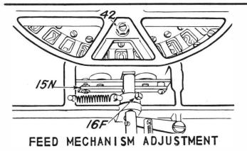
Proper spring tension on lower feed wheels is set at the factory. If necessary to remove collar be sure that set screw 16F is seated in original position or slightly in the direction of increased tension.
