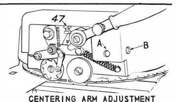
RELEASE LOCKSCREW. Look thru hole marked A to observe position of screw slot. Insert screwdriver and loosen screw 1/2 turn counterclockwise.
