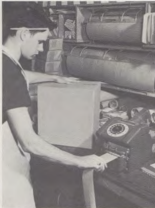
This food shipper found the Electric DIAL-TAPER to be a big improvement over hand-operated machines while saving 15 seconds per unit taped and also eliminating wasted tape.
